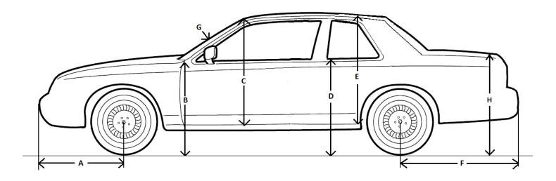
A Centerline of front wheels to forward most point of front bumper. B Rear top edge of fender to ground. (at
