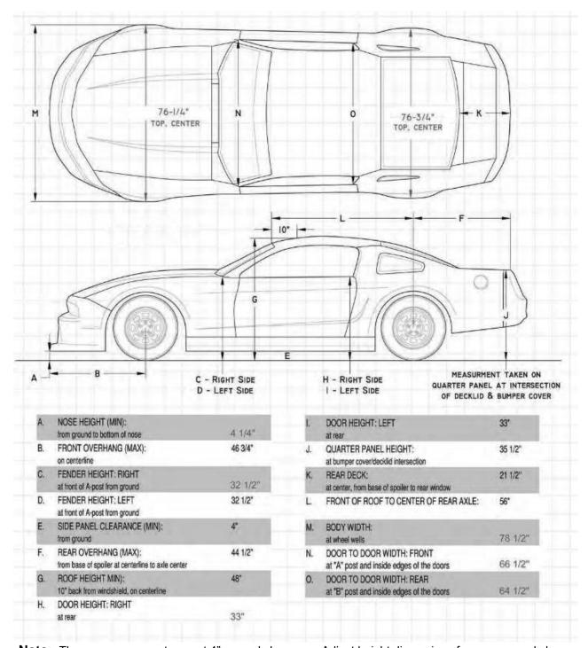
**Note:** These measurements are at 4" ground clearance. Adjust height dimensions for your ground clearance.
