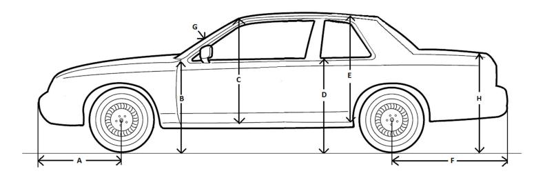
A Centerline of front wheels to forward most point
